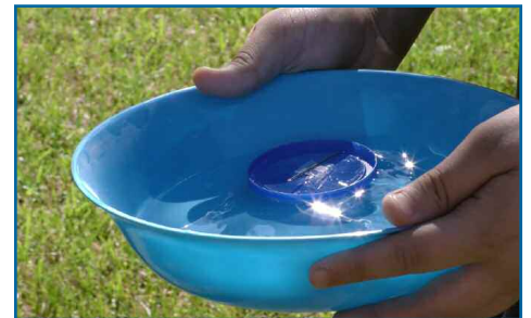
This compass made by Manalapan students as part of the REACH pilot uses the same components as 14th-century compass: a bowl, a float, and magnetized needle.
